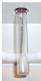
Figure 3: 16 mL Single-shot™ amino acid apparatus
